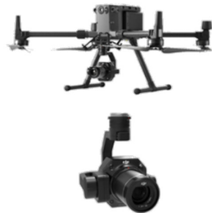
Figure 2. DJI M300RTK UAV with Zenmuse P1 gimbal camera.
