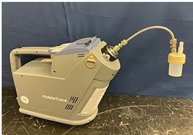
Figure 9. Non-contact detection of fentanyl by a field-portable ion mobility spectrometer [169]. Reprinted from [169], Copyright (2018), with permission Wiley and Sons.
