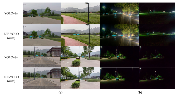
Figure 12. Visualization of small-scale pedestrian-detection results under different illumination on the Jetson Orin NX platform. (a) Day. (b) Night.
