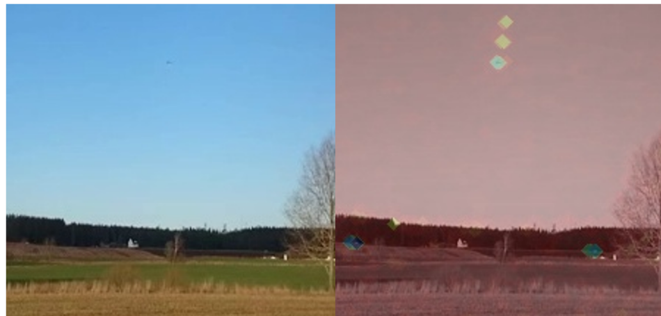
Figure 6. Image enhancement during annotation allows the discovery of additional tiny objects in the dataset that could otherwise easily be missed. Left: the original image, where the small objects are barely visible and thus very difficult to annotate. Right: the colored overlay based on frame differences, highlighting the small objects and facilitating more accurate annotation.
