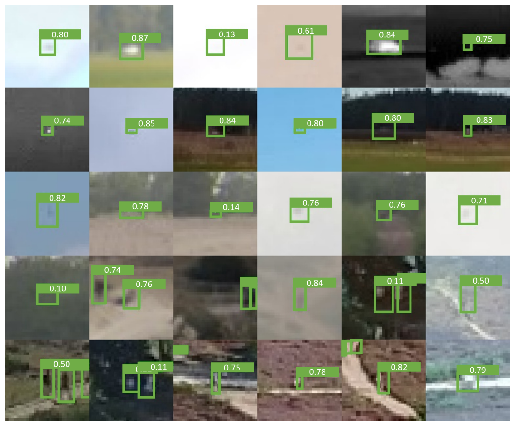
Figure 11. Example detections from the proposed Temporal-YOLOv8 model. These crops have been resized to four times their original size. The value drawn in each bounding box refers to the confidence of the prediction.
