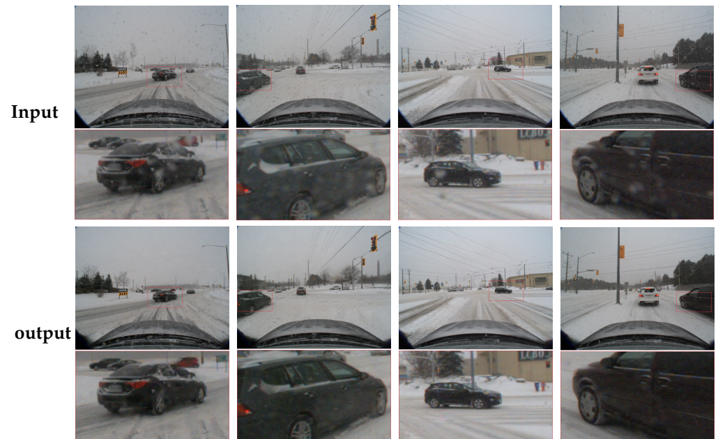
Figure 2. TKLMR snowflake removal results. Input is the input raw image and Output is the result after applying the TKLMR severe weather removal algorithm.
