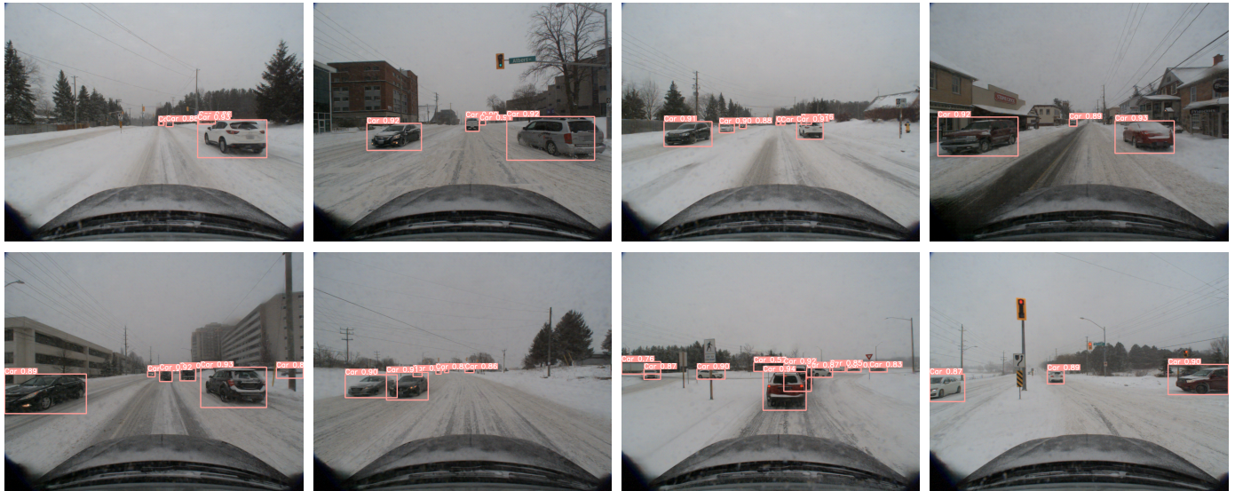
Figure 8. Results of 2D object detection on the validation set of the CADC public dataset. The red box indicates the object position predicted by our algorithm, and the corresponding number indicates the confidence score.
