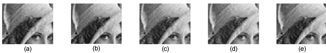
Figure 9. Details of reconstructed Lena: (a) Gaussian random measurement matrix, (b) our proposed measurement matrix, (c) random binary measurement matrix, (d) random symmetric measurement matrix, and (e) bipartite graph measurement matrix.
