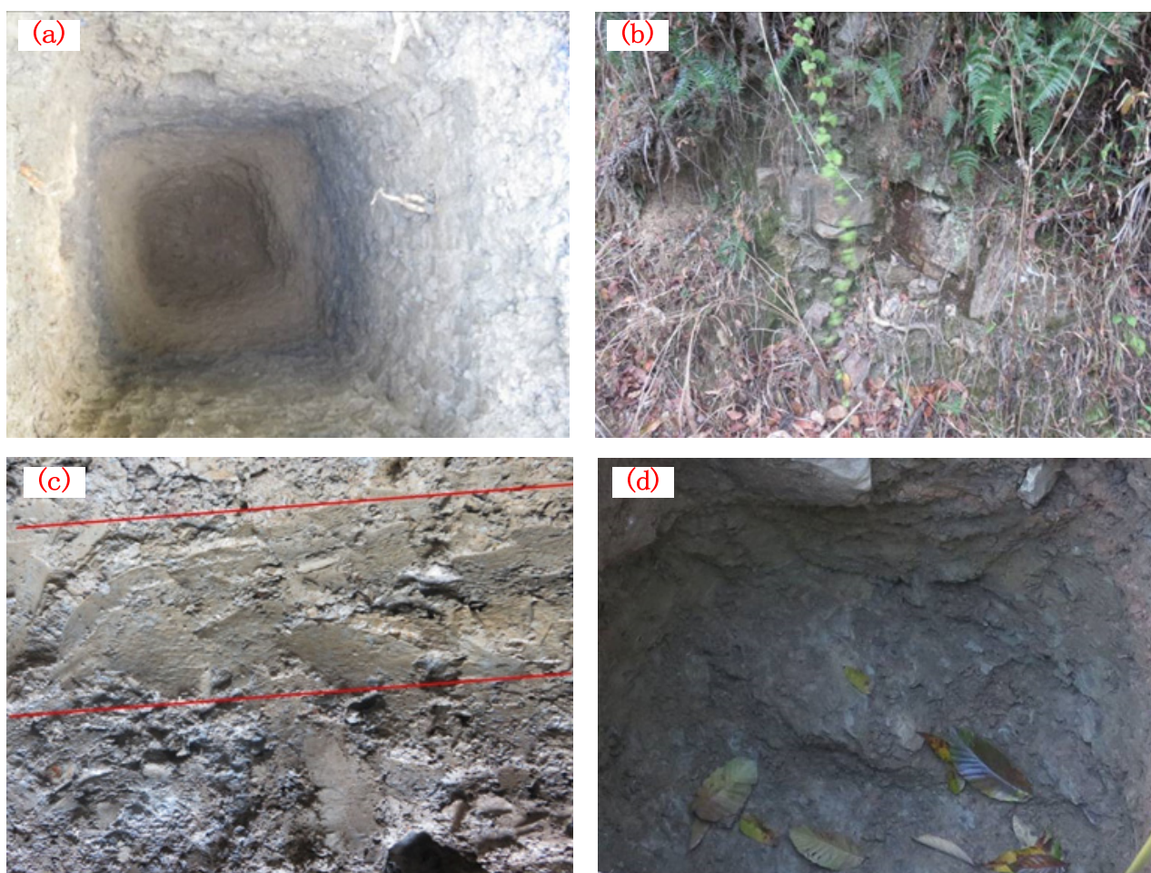
Figure 2. (a) Exploratory pit, (b) Quaternary residual layer, (c) the Upper Silurian Gauze Hat Group, (d) the Middle Silurian Luojiaping Group.
