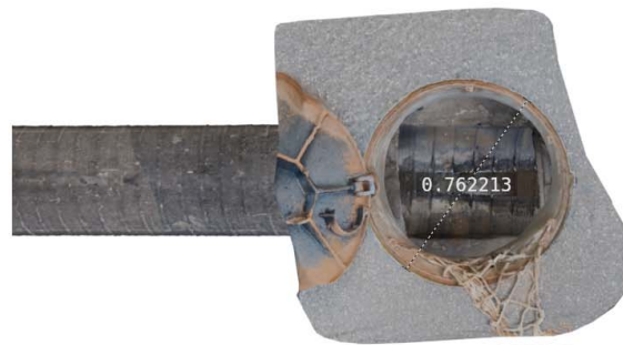
Figure 25. Inspection well bore diameter measurements.
