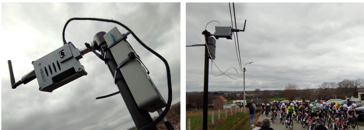
Figure 1. Hardware setup of a STRADA device during junior cycling race field test in Sint-Maria-Lierde.
