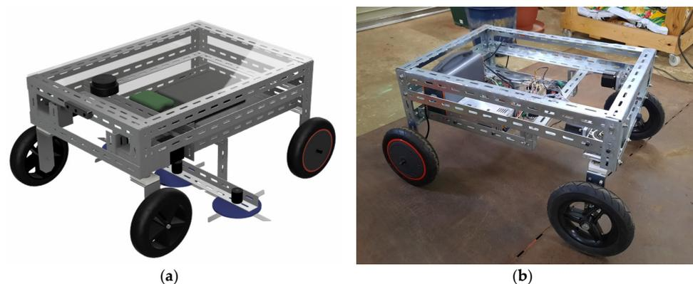
**Figure 11.** The autonomous robotic weeder preparation for the orchard, especially at the intrarow area: (a) 3D model of the final product and (b) robotic weeder in progress during reconstruction.
