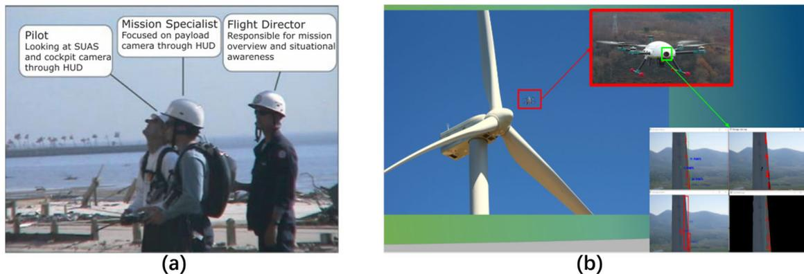
**Figure 10.** Manually operated and automatic UAVs. (a) Flight team with mission responsibilities noted, adapted with permission from Ref. [182], copyright ©2009 Wiley Periodicals LLC; (b) WEGOOI project: Inspection services for wind turbines, damage assessment and repair recommendation reports using artificial intelligence and reviewed by engineers, image from <https://aleriontec.com/en/project/weggoi/> accessed on 20 December 2023 (Ref. [184]).
