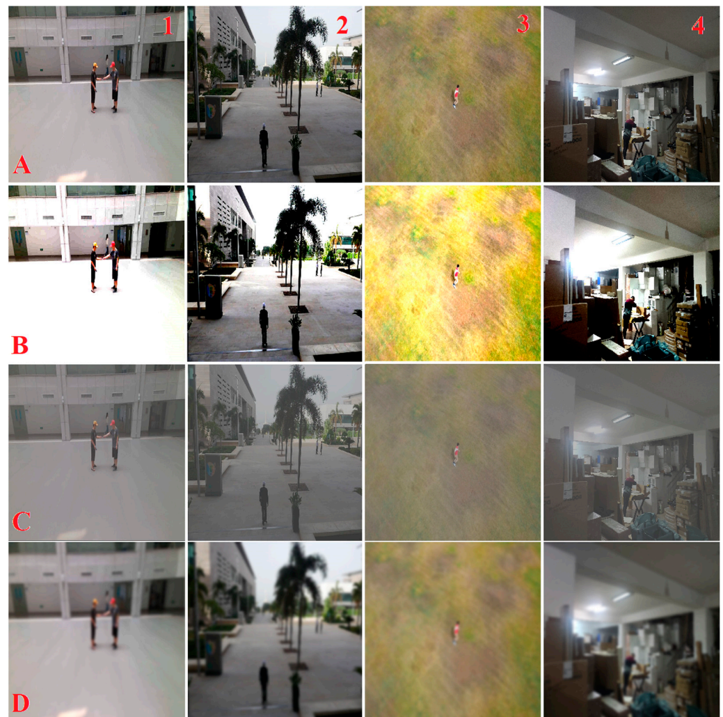
Figure 4. UAVHuman Dataset (1), UAV123 Dataset (2–3), Own Collection (4). Original image (A), increased brightness (B), decreased contrast (C), and blurred (D).
