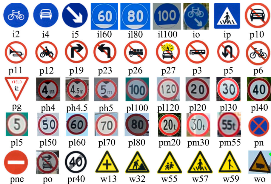
Figure 12. The 45 traffic sign classes with more than 100 instances in the TT100K dataset.
