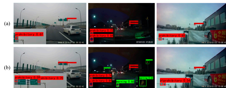
Figure 14. Ablation results for FMEM tested on the CCTSDB2021 dataset. (a) YOLOv7; (b) YOLOv7 + FMEM.
