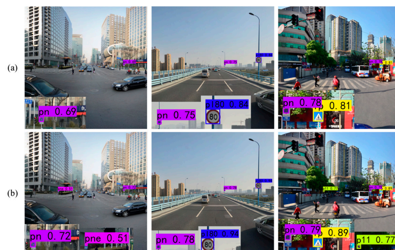
Figure 21. Comparison results of YOLOv7 and YOLOv7-TS tested on the TT100K dataset. (a) YOLOv7; (b) YOLOv7-TS.
