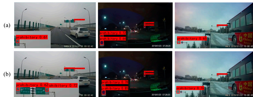
Figure 18. Ablation results for DFEM tested on the CCTSDB2021 dataset. (a) YOLOv7; (b) YOLOv7 + DFEM.
