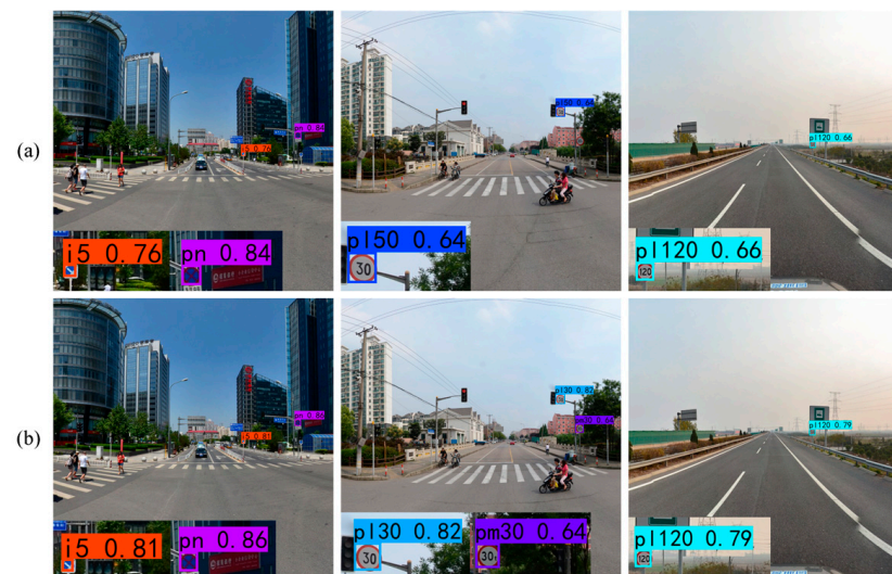
Figure 19. Ablation results for DFEM tested on the TT100K dataset. (a) YOLOv7; (b) YOLOv7 + DFEM.
