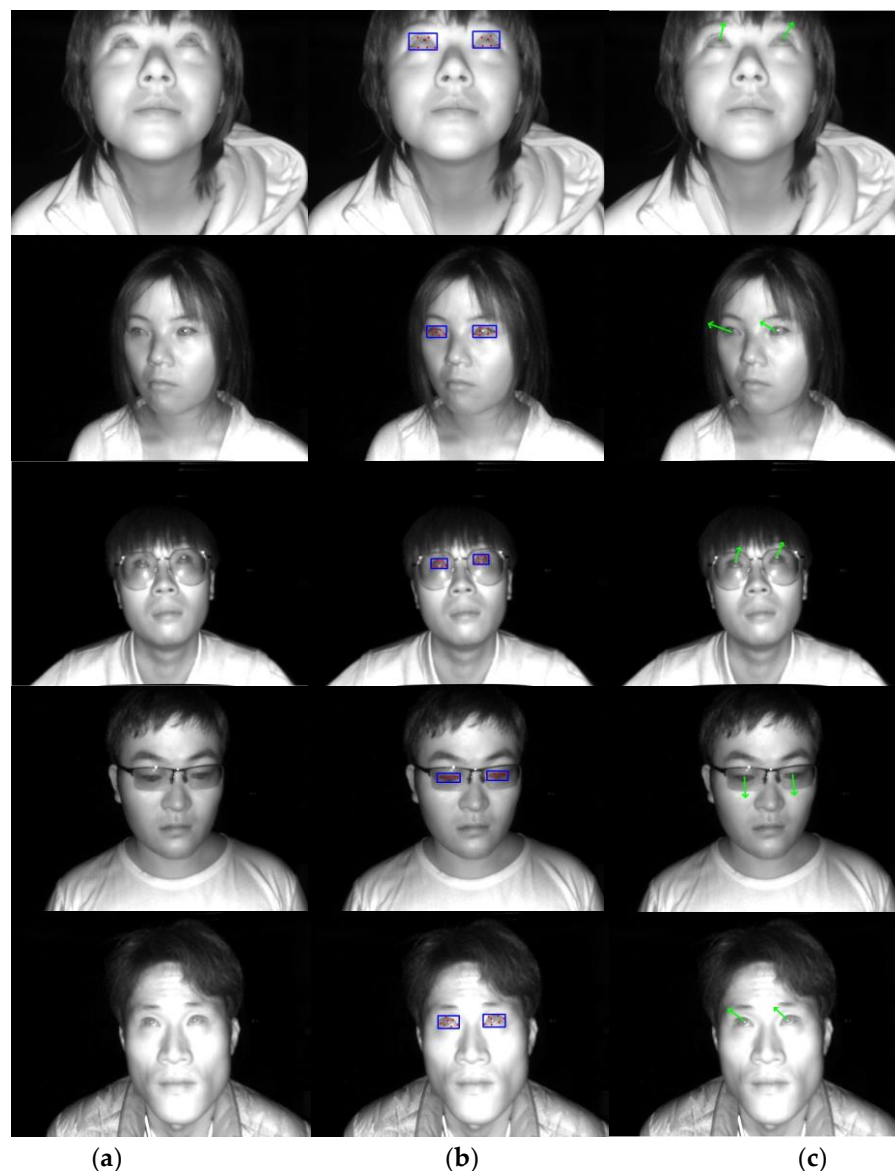
Figure 16. Results of the subject's gaze detection. Column (a) presents the original gaze images of the subject, column (b) shows the results of eye landmark detection based on YOLOv8, and column (c) visualizes the subject's gaze direction. The green arrow indicates the gaze direction detected by our model.
