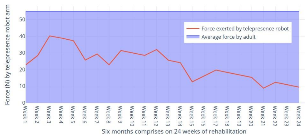
Figure 11. Comparison of force exerted by the robotic arm as compared to normal adults.
