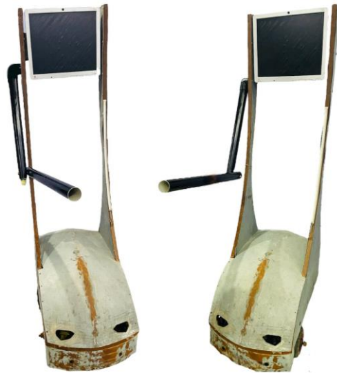
Figure 3. Telepresence robot with a robotics arm for elbow flexion exercises.
