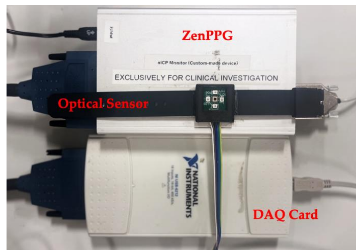
Figure 1. Optical wearable sensor connected to the ZenPPG processing system and the Data Acquisition Card (DAQ).
