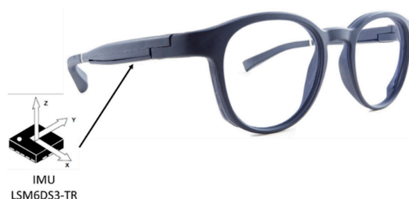
Figure 1. Placement of the Inertial Measurement Unit (IMU) in the temple of the smart eyeglasses.
