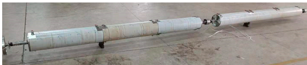
Figure 3. Hydrogen permeation test autoclave.
