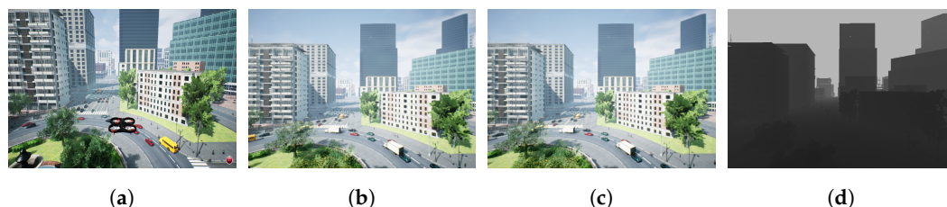
Figure 5. An example of an AirSim city environment showing the following: (a) the FPV view in the simulator where the drone is hovering, (b) RGB image from the simulated left camera mounted on the drone, (c) RGB image from the simulated right camera, and (d) depth image from the simulated depth sensor where objects closer to the depth camera appear darker. (a) AirSim simulator; (b) left camera image; (c) right camera image; (d) Depth image.
