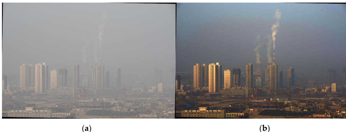
Figure 1. Dark channel defogging effect: (a) images with sky areas; (b) result of dark channel algorithm.
