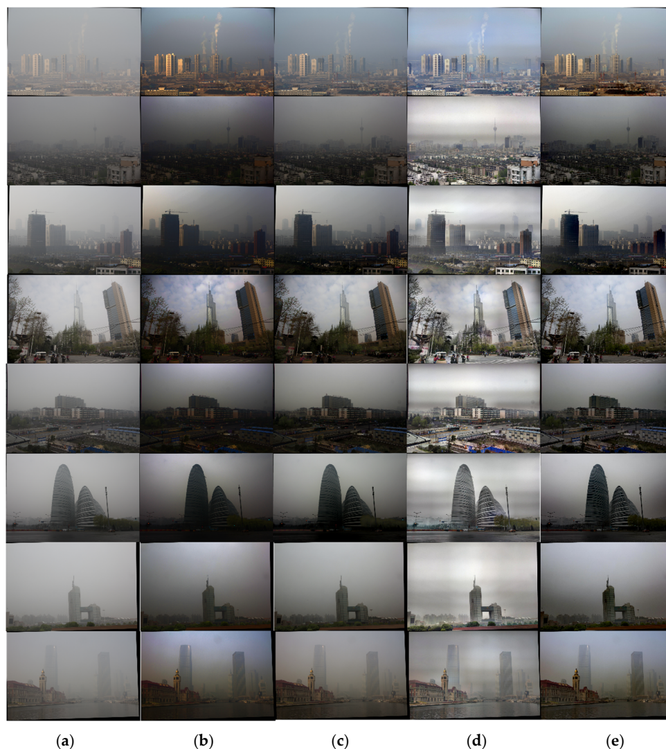
Figure 16. Comparison of image defogging effects: (a) original foggy image; (b) defogging results of He's algorithm; (c) defogging results of Zhu's algorithm; (d) defogging results of the Retinex algorithm; (e) results of the proposed algorithm defogging.
