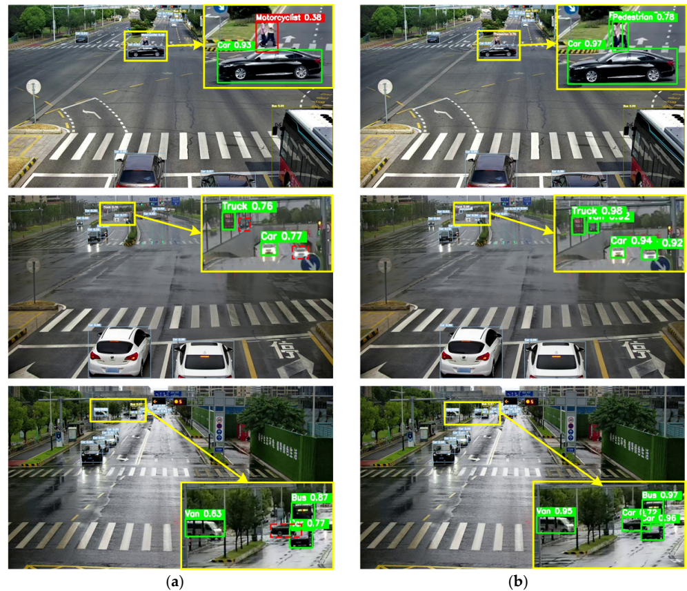
Figure 10. Visualization of algorithm model detection results on the IVODC dataset. (a) YOLOv7-tiny; (b) PDT-YOLO. All of the key areas with yellow boxes are enlarged and displayed. The red solid line indicates false detection, the red dashed line indicates missed detection and the green line indicates correct detection.
