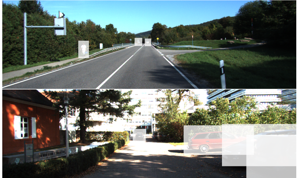
Figure 4. Previous depth completion loss calculations required assessing the valid depth areas across the entire image. In this paper, we leverage target boxes derived from object detection to generate masks (represented by the semi-transparent areas in the image) for the isolated computation of depth completion loss in regions containing targets.
