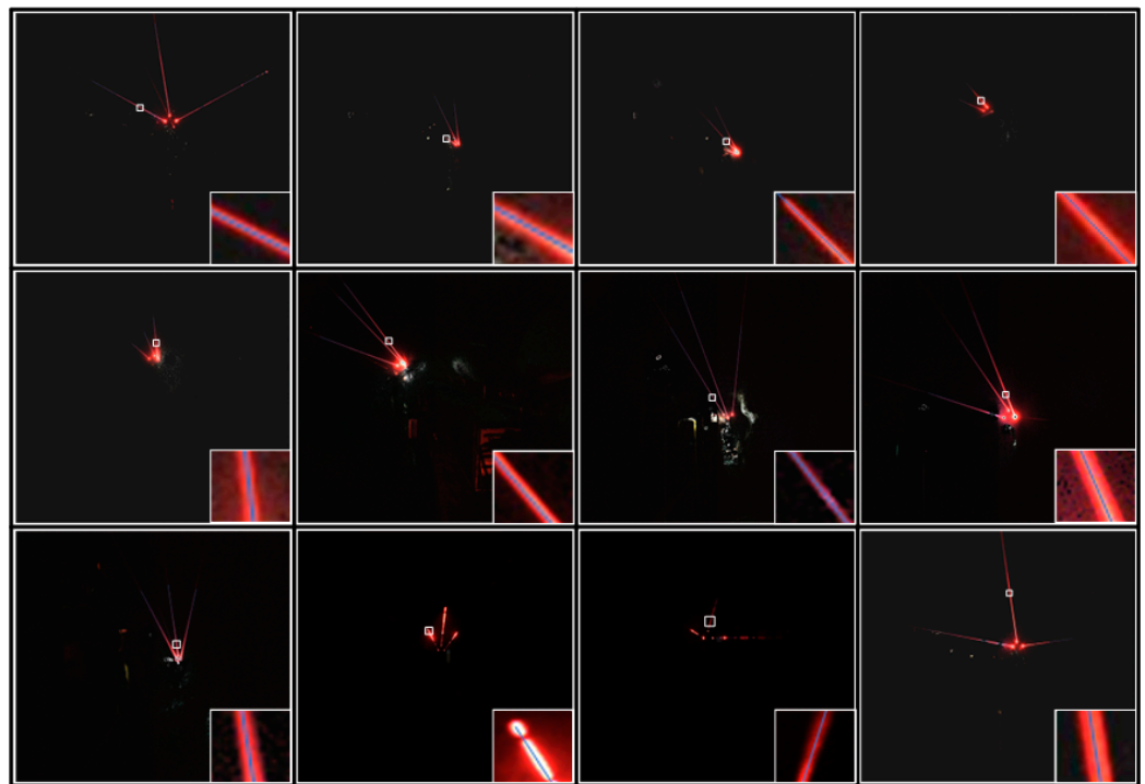
Figure 14. The center line fitting results of multi-laser beams.
