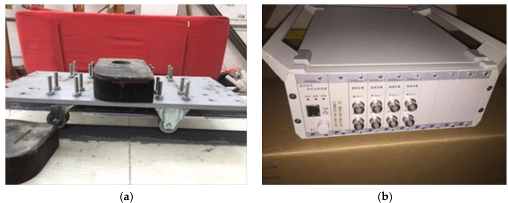
Figure 15. Experimental setup: (a) model car, (b) DH5920 dynamic test system.
