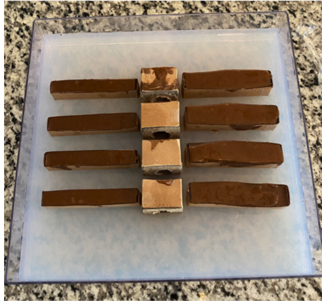
Figure 1. Layout of epoxy-based features within the supporting tray prior to complete filling with an agarose gel—the tray is partially filled with gel, as shown, to elevate the rectangular blocks to the mid-height of the tray. The central square blocks extend from the tray bottom to \sim 4.0 cm of height above the tray floor. Note the holes drilled through the central square blocks.
