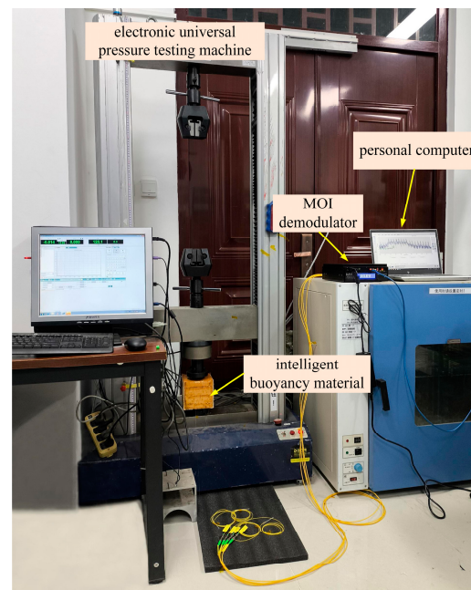
Figure 12. Compression experimental of intelligent buoyancy material.
