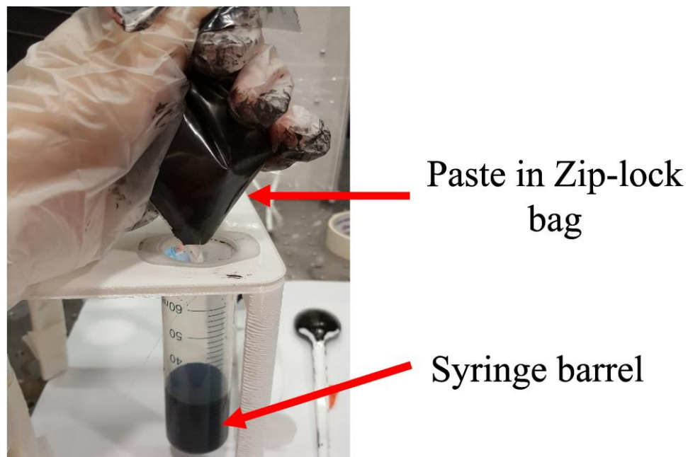
Figure S1. The filling of carbon paste into the syringe barrel. To avoid bubbles, the paste is squeezed into the syringe barrel through a 2 mm diameter small hole cut on the corner of a zip-lock bag.
