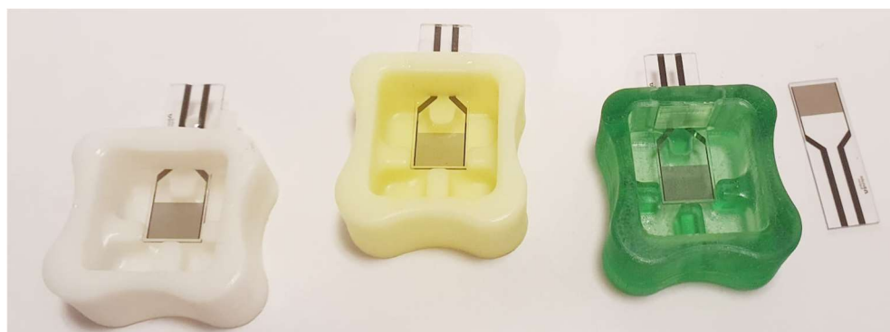
Figure 2. The cuvette and electrode setup in the biosensor and free IDE used and designed within the measurements.
