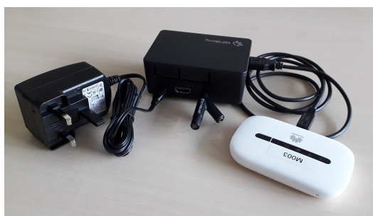
Figure 1. Bedside cough monitor: left: adapter; mid: single-board computer and microphone; and right: dongle.
