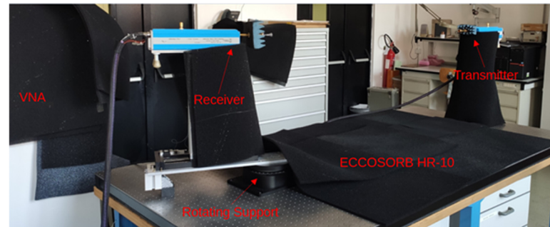
Figure 5. Picture of the measurement setup.
