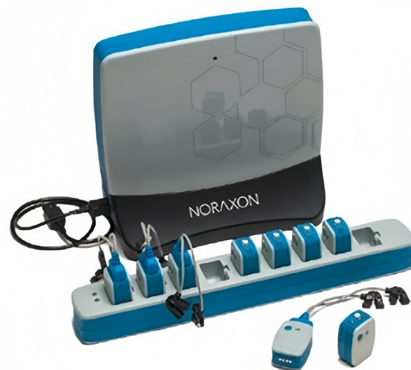
Figure 2. Surface EMG testing and analysis system.
