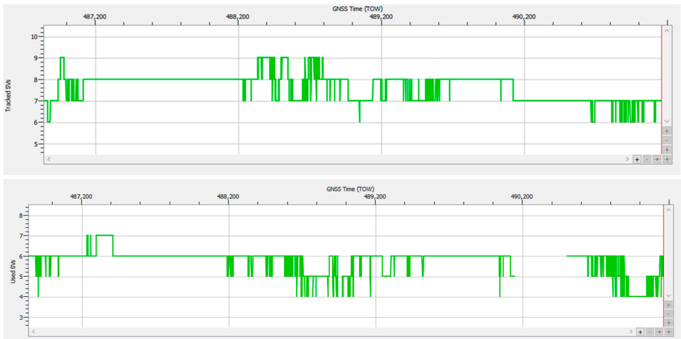
Figure 14. Test drive #15: Upper half —number of Galileo satellites in track vs. time during; lower half —number of Galileo satellites in PVT calculation vs. time.
