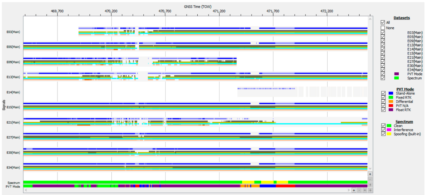
Figure 10. Signals of Galileo satellites tracked vs. time, test drive #4. Color legend for signal bands: blue—E1, dark green—E6, light green—E5a, cyan—E5b, pink—E5.
