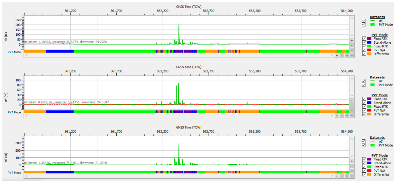
Figure 22. Positional accuracy: standard deviation time plot for test drive #13, case study #3 (obstructions due to environment).
