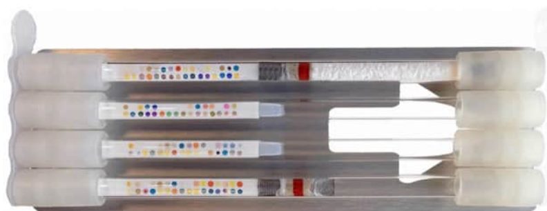
Figure 22. Colorimetric sensor array cartridge with integrated desiccant. There are 4 channels for airflow, each containing 32 sensor elements. The top channel contains a desiccant and oxidizer. Reprinted from ref 114 with permission of the American Thoracic Society. Copyright 2015 American Thoracic Society.
