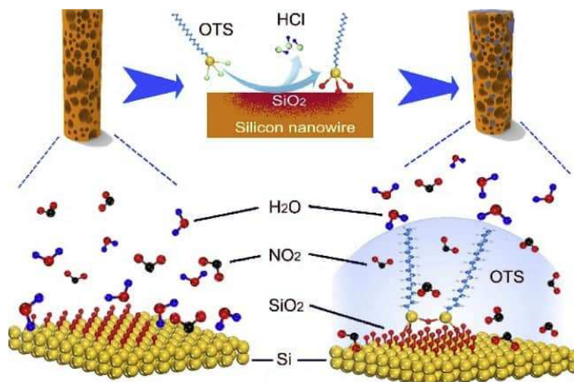
Fig. 1. Schematic illustration of construction of OTS-modified porous SiNWs for NO 2 detection under high humidity condition.
