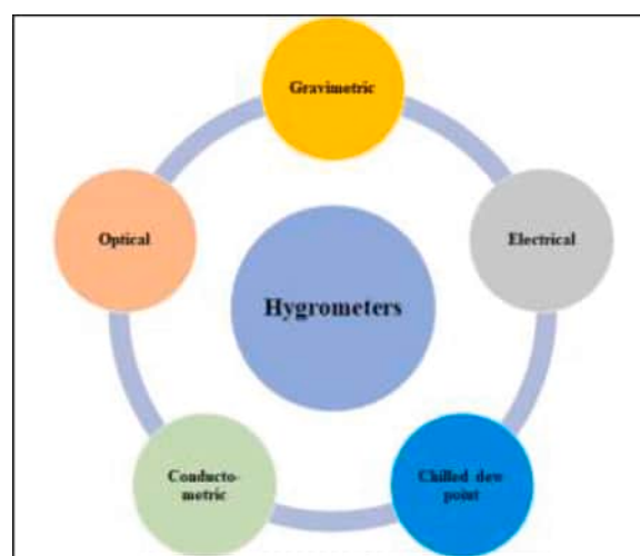
Fig. 5. Classification of humidity sensors based on the change in the physical properties with change in the humidity.
