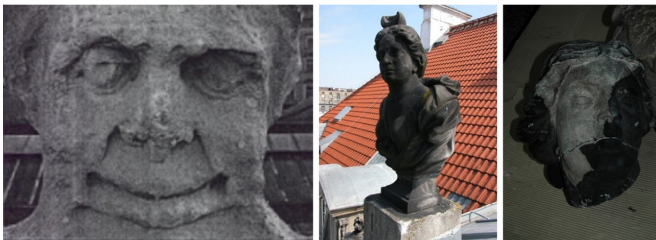
Figure 1. Illustration of destructive influence of acid rains on sandstone sculptures: a) Drapper's Hall in Cracow (1995); b) bust at Czapski Palace, Warsaw, seat of Academy of Fine Arts; c) woman's head during laser cleaning.
