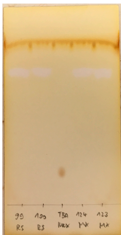
Figure 3. Iodine-stained TLC from the tetrabutylammonium (TBA) test showing the reference solution 0.1 mg/mL in the middle and respective final solutions from TRACERlab MX ( left ) and mosaic-RS ( right ).
