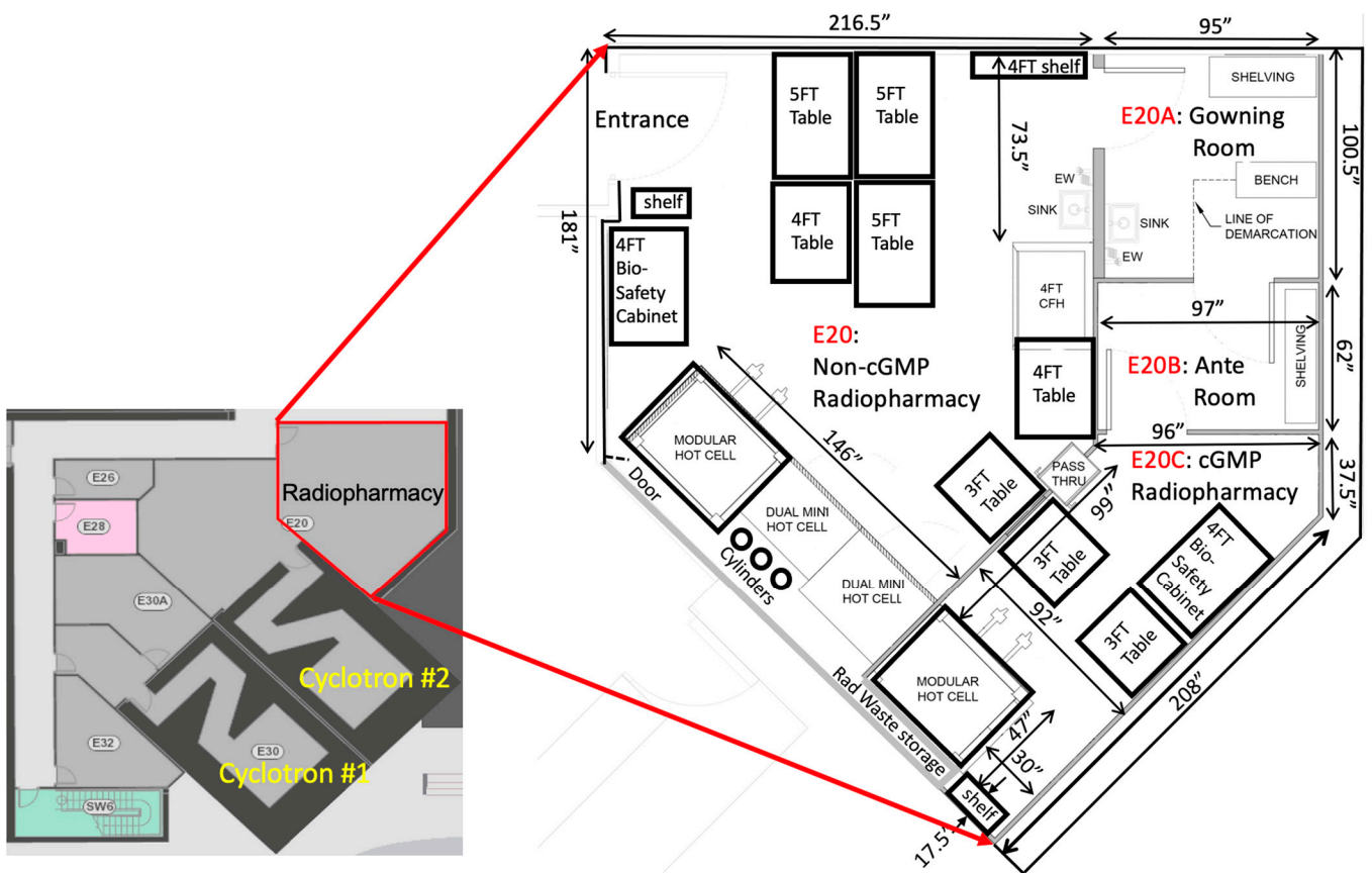
Figure 1. Schematic diagram of the radiopharmacy facility layout, including the radiochemistry laboratory (E20), cleanroom system (E20A-C), as well as the hot cells, biosafety cabinets, tables, and shelves. The vaults and cyclotron locations are indicated in the inset and are adjacent to the radiopharmacy facility.
