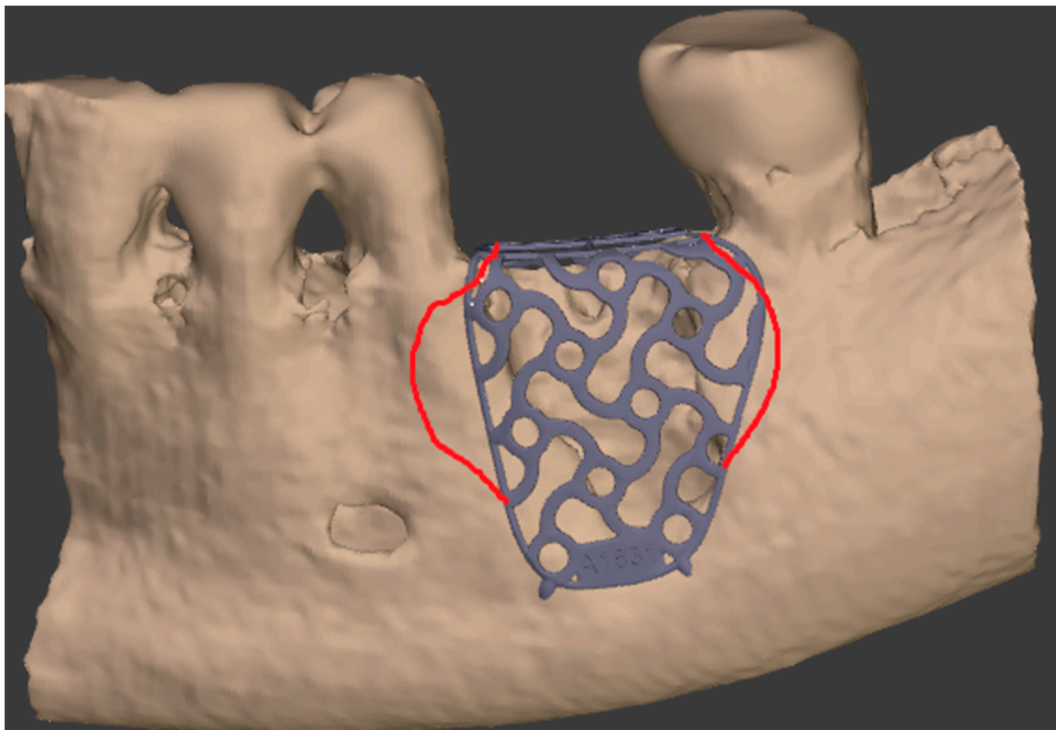
Figure 1. The digital planning of the custom made titanium mesh with the feedback corrections.
