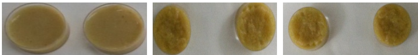
Figure 1. Pictures of biocomposites made with 2% polymer and 10% nutrients. (Right) agar; (center) alginate; (left) \kappa -carrageenan.
