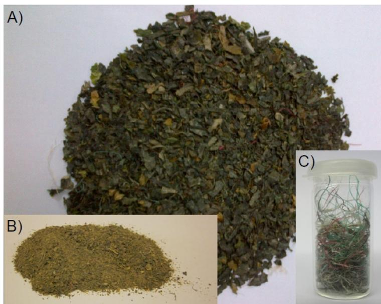
**Figure 8.** *Laminaria japonica* waste substrate: Dry and native *Laminaria japonica* waste material as obtained from Qingdao CoDo International Limited, Qingdao, China (a) containing plastic braids (c). For laboratory use, the biomaterial was shredded and sieved to a particle size of  $<0.5\text{ cm}$  (b).
