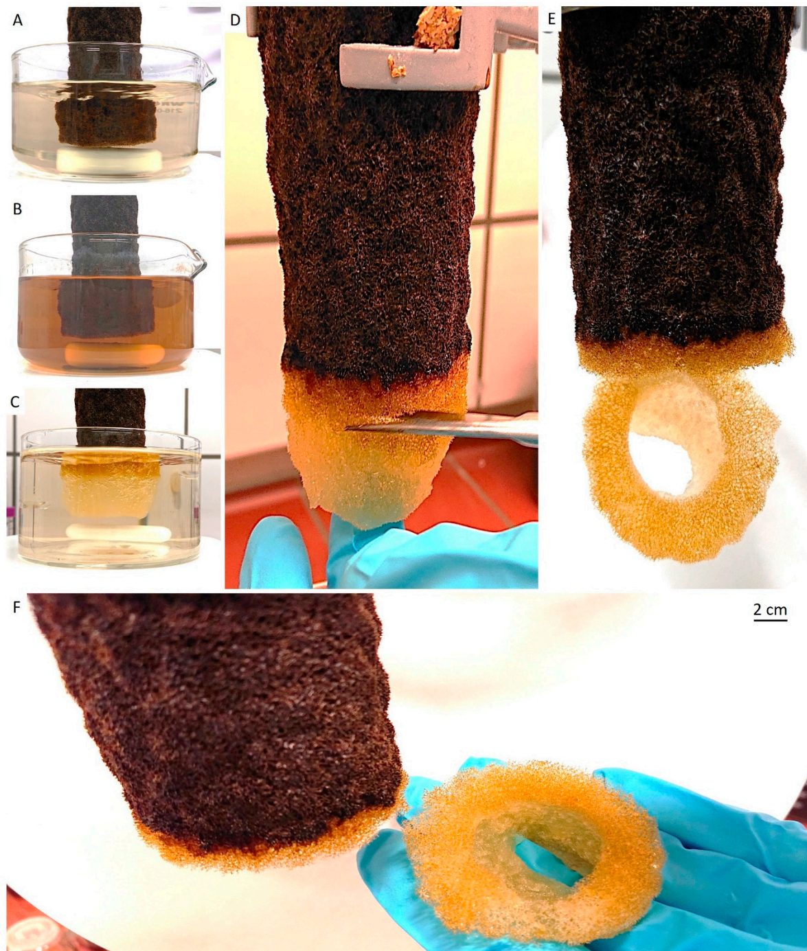
Figure 3. Step-by-step isolation of selected fragment of 3D tubular chitin scaffold from dried A. archeri segment. In step I, water-soluble salts were removed by pretreatment of the sponge skeleton with distilled water in the beaker placed on a magnetic stirrer (A) for 6 h. Afterward, in step II, the sponge was treated with 2.5 M of NaOH solution during 24 h, for deproteinization and depigmentation (B). In step III, the 3D scaffolds were treated with 20% acetic acid for 24 h, to remove residual calcium and magnesium carbonates, followed by washing with distilled water up to pH 6.8 (C). Steps II and III were repeated twice to obtain tubular scaffolds (D,E), which were cut off from the sponge and used for further studies (F).
