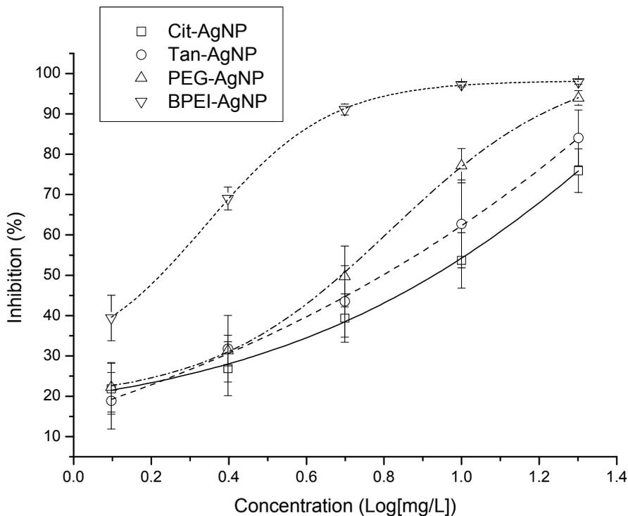
**Figure S6.** Fitted sigmoidal dose-response curves for the 4 different surface-coated AgNPs with luminescent bacteria strain #6 (*Photobacterium phosphoreum*, NCIMB 30271) of the LumiMARA system.
