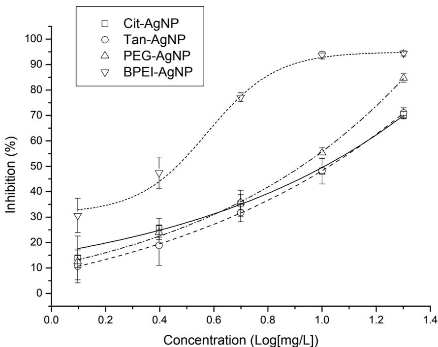
**Figure S9.** Fitted sigmoidal dose-response curves for the 4 different surface-coated AgNPs with luminescent bacteria strain #9 (*Vibrio fischeri*, NCIMB 30274) of the LumiMARA system.
