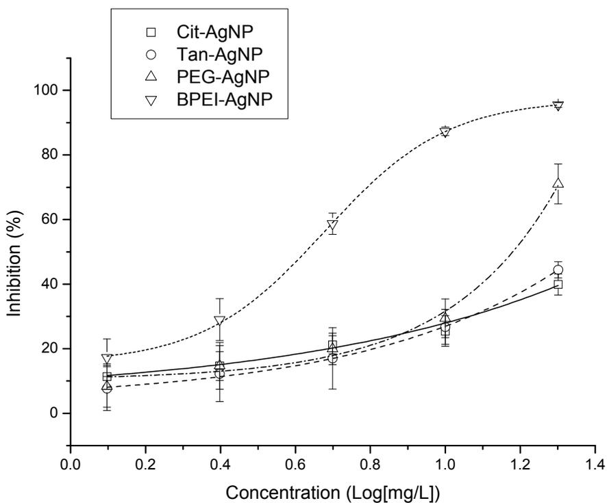
**Figure S7.** Fitted sigmoidal dose-response curves for the 4 different surface-coated AgNPs with luminescent bacteria strain #7 (*Vibrio harveyi*, NCIMB 30272) of the LumiMARA system.
