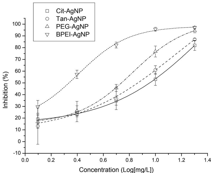
**Figure S4.** Fitted sigmoidal dose-response curves for the 4 different surface-coated AgNPs with luminescent bacteria strain #4 (*Photobacterium leiognathi*, NCIMB 30269) of the LumiMARA system.
