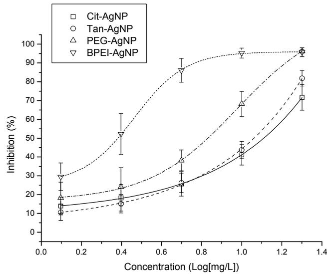
**Figure S2.** Fitted sigmoidal dose-response curves for the 4 different surface-coated AgNPs with luminescent bacteria strain #2 (*Photobacterium phosphoreum*, NCIMB 30267) of the LumiMARA system.
