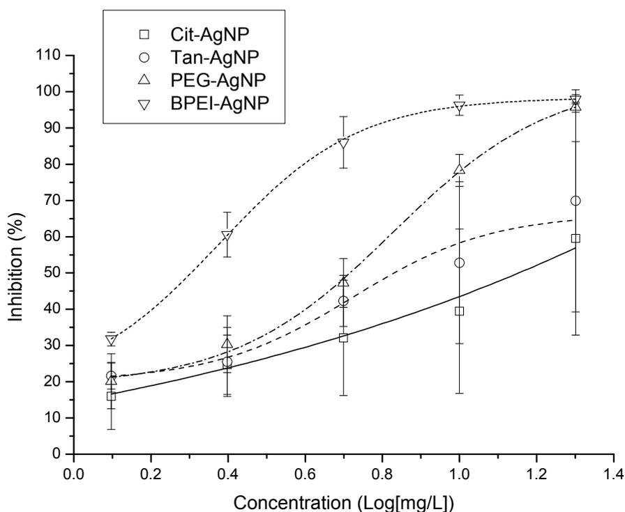
**Figure S5.** Fitted sigmoidal dose-response curves for the 4 different surface-coated AgNPs with luminescent bacteria strain #5 (*Photobacterium phosphoreum*, NCIMB 30270) of the LumiMARA system.
