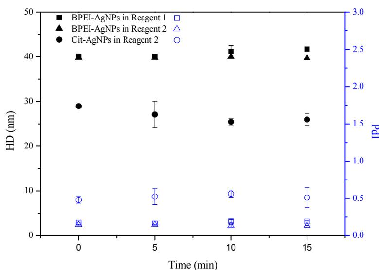
**Figure S13.** Time-dependent changes in hydrodynamic diameter (HD) and polydispersity index (Pdl) for Cit-AgNPs and BPEI-AgNPs during their exposure time in tested medium.
