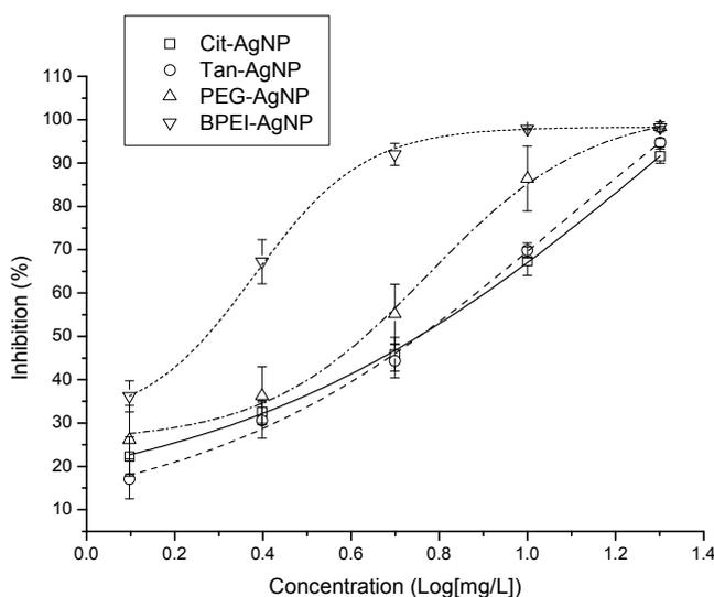
**Figure S1.** Fitted sigmoidal dose-response curves for the 4 different surface-coated AgNPs with luminescent bacteria strain #1 (*Photobacterium leiognathi*, NCIMB 30266) of the LumiMARA system.
