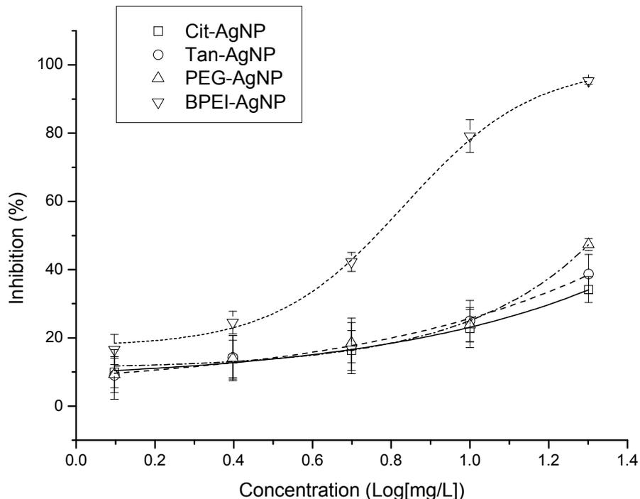
**Figure S8.** Fitted sigmoidal dose-response curves for the 4 different surface-coated AgNPs with luminescent bacteria strain #8 (*Vibrio harveyi*, NCIMB 30273) of the LumiMARA system.
