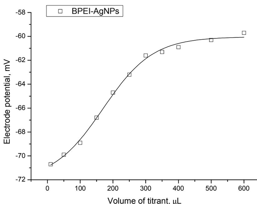
**Figure S12.** Titration curve of BPEI-AgNPs for determining the free silver ions released from these nanoparticles; titration of iodide ( $1.02 \times 10^{-4}$  mM) against 0.015  $\mu$ L volumes of AgNPs solution (4.71 mg/L as mass concentration of silver).
