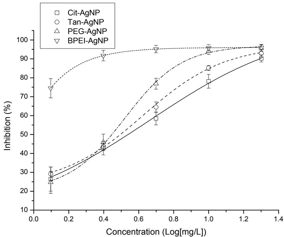
**Figure S3.** Fitted sigmoidal dose-response curves for the 4 different surface-coated AgNPs with luminescent bacteria strain #3 (*Vibrio fischeri*, NCIMB 30268) of the LumiMARA system.
