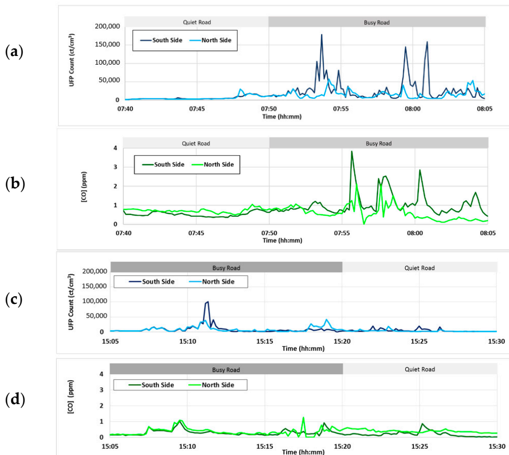
Figure 3. Example time series of exposure during the morning Walking School Bus (WSB) for (a) UFP (ultrafine particle) and (b) CO and the afternoon (c) UFP and (d) CO. The participant walking on the north side of the street (high traffic side during the morning rush hour and low in the afternoon) is shown in the darker color.
