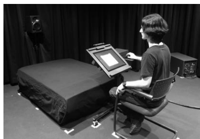
Figure 4. Laboratory setup in AuraLab at Empa, with the listening test program (graphical user interface) displayed on the screen and a porous floor absorber between loudspeaker and participant. One of the two subwoofers is visible on the right side.
