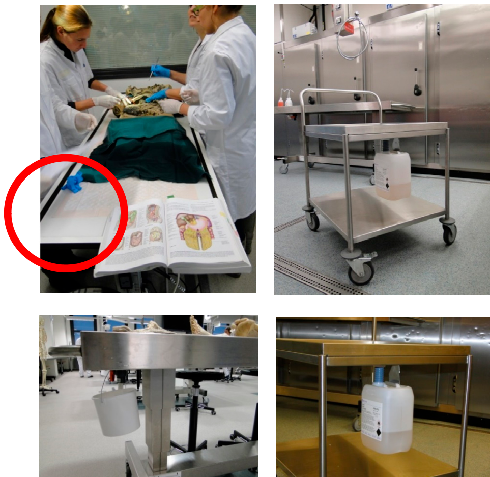
Figure 4. Before (left panels) and after (right panels) elimination of disposable absorbent sheets (red circle) and introduction of a containment system (instead of an open bucket) to collect leaking formalin residue (T-2 in Table 2).
