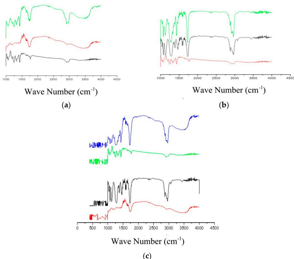
**Figure 5.** FT-IR spectra of different PIMs and their constituents. (a) PVC/poly( $\beta$ -cyclodextrin) membrane (green), PVC (black) and poly( $\beta$ -cyclodextrin) (red). (b) PVC/DBP membrane (green), PVC (red) and DBP (black). (c) PVC/DBT/poly( $\beta$ -cyclodextrin) membrane (blue), PVC (green), DBP (black) and poly( $\beta$ -cyclodextrin) (red). Each measurement was made in triplicate.
