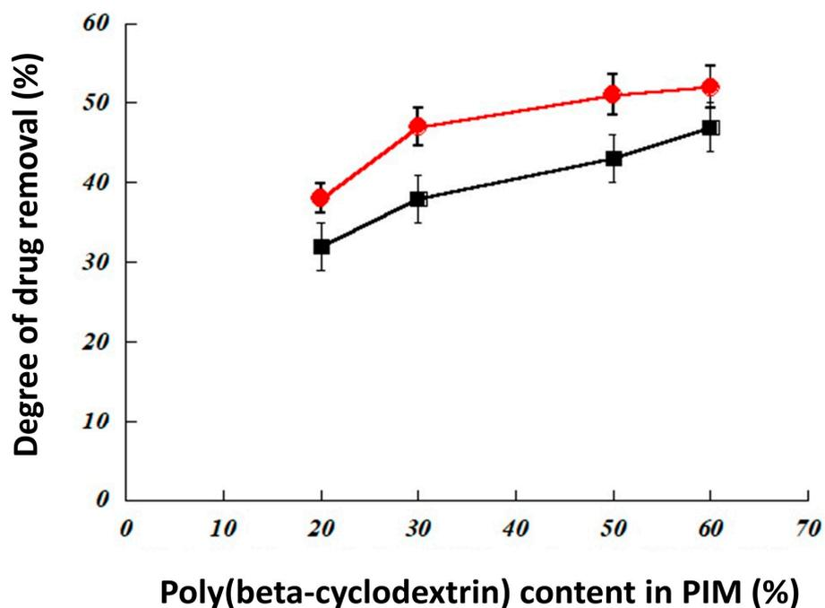
**Figure 8.** Influence of poly( $\beta$ -cyclodextrin) content in the PVC/DBP/poly( $\beta$ -cyclodextrin) membrane on the extraction of residual drug in wastewater. Two drugs were tested at an initial concentration of 10 ppm: ibuprofen (red circles) and progesterone (black squares). The extraction process was performed over 6 h. Each assay was performed in triplicate.
