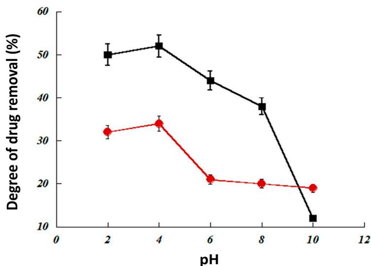
**Figure 9.** Influence of pH on extraction of residual drug in wastewater. Two drugs were tested at an initial concentration of 10 ppm: ibuprofen (red circles) and progesterone (black squares). The extraction process was performed over 6 h. Each assay was performed in triplicate.
