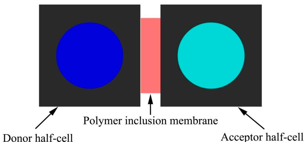
**Figure 2.** Experimental setup for the pharmaceuticals extraction with Polyvinyl chloride/dibutylphthalate/poly( $\beta$ -cyclodextrin) membrane extraction cell. In the donor half-cell there is initially 60 mL of aqueous solution of the drug (ibuprofen or progesterone) at 10 ppm. Sample for measurements were taken from acceptor half-cell.
