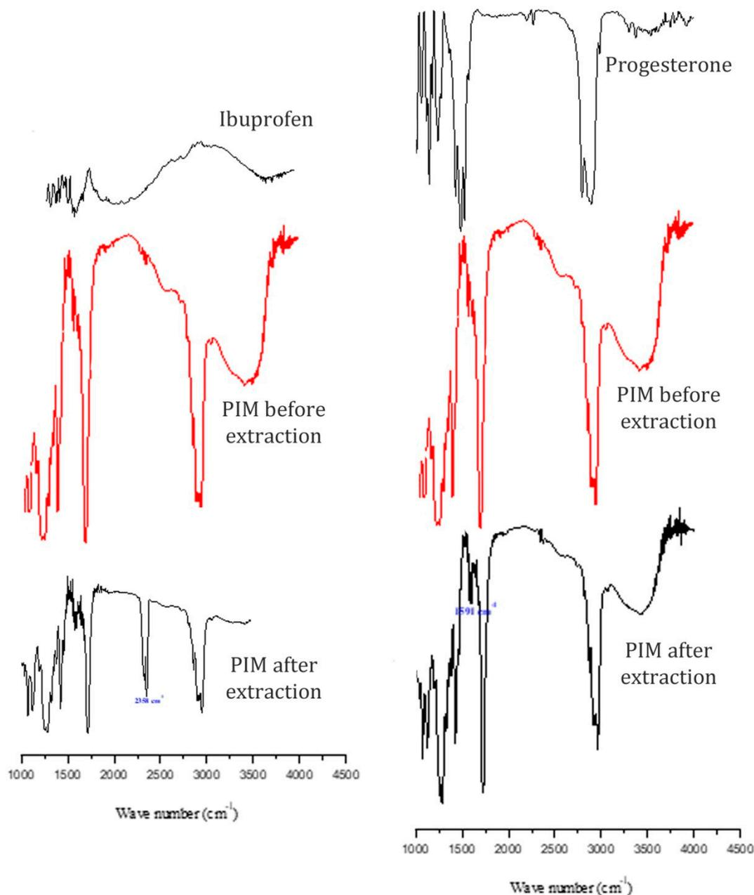
**Figure 6.** FT-IR spectra of different PIMs before and after extraction of ibuprofen and progesterone.
