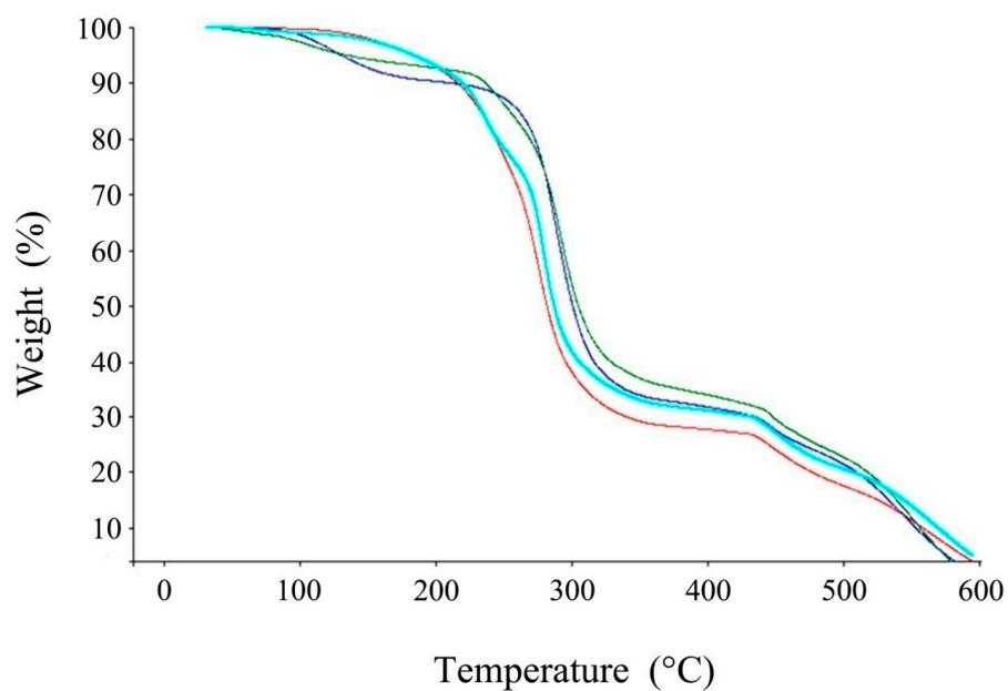
**Figure 4.** TGA profiles of PVC (dark blue) and different polymer inclusion membranes: PVC/DBP (red), PVC/poly( $\beta$ -cyclodextrin) (green) and PVC/DBP/poly( $\beta$ -cyclodextrin) (light blue). Each experiment was performed in triplicate.
