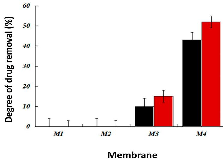
**Figure 7.** Influence of membrane composition on extraction of residual drug in wastewater. Different membranes were tested: PVC (M1), PVC/DBP (M2), PVC/poly( $\beta$ -cyclodextrin) (M3) and PVC/DBP/poly( $\beta$ -cyclodextrin) (M4). Two drugs were tested at an initial concentration of 10 ppm: ibuprofen (red circles) and progesterone (black squares). The extraction process was performed over 6 h. Each assay was performed in triplicate.
