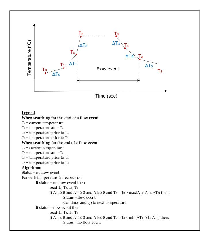
Figure S1. Flow/flushing event algorithm.
