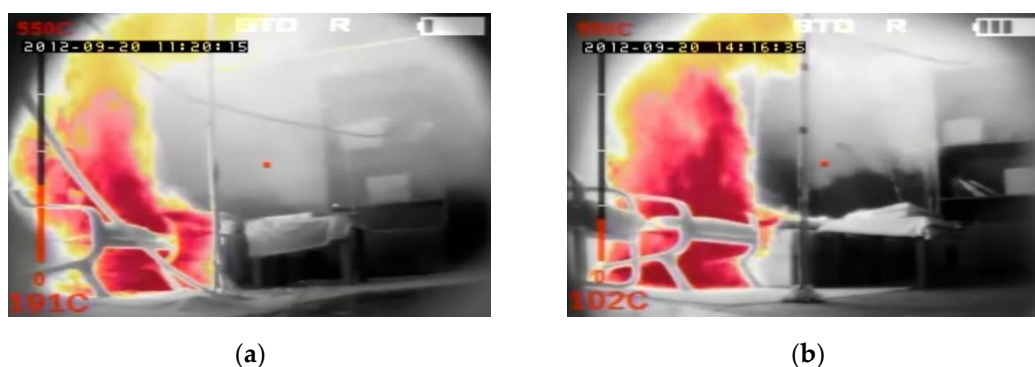
Figure 14. Frames from the movie recorded with thermal imaging camera at 180 s of the fire in the: (a) sealed apartment; (b) unsealed apartment.
