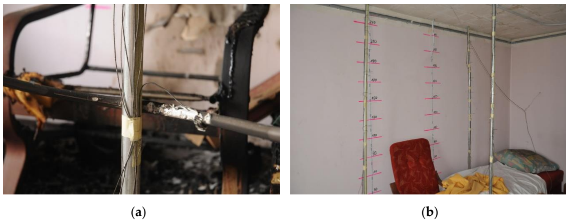
Figure 8. Pictures of: (a) a thermocouple T3 placed by the armchair after fire test; (b) a scale with height levels on the wall.
