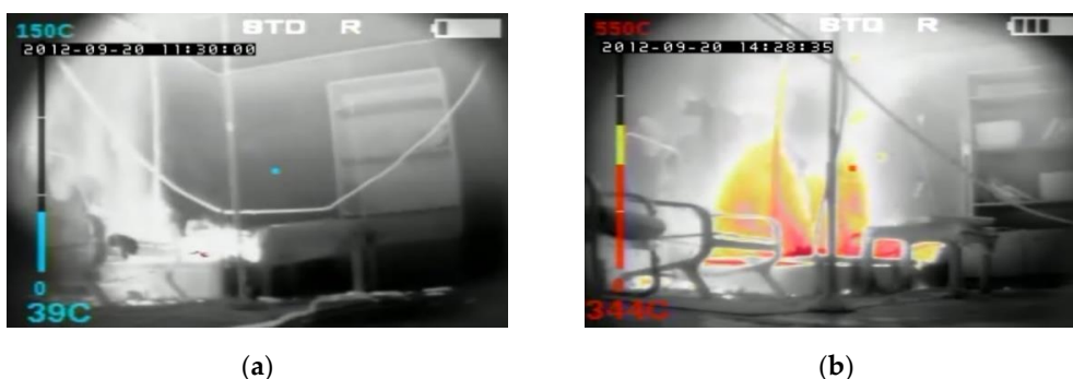
Figure 16. Frames from the movie recorded with a thermal imaging camera at 900 s of the fire in the: (a) sealed apartment; (b) unsealed apartment.
