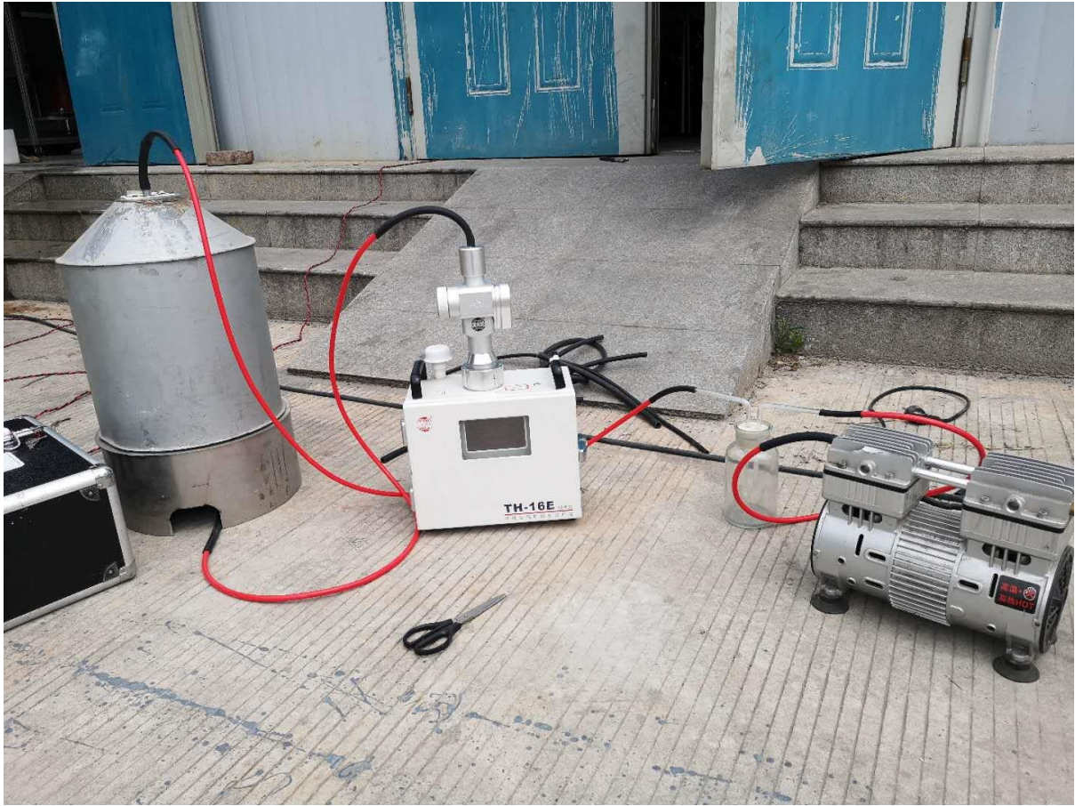
Figure S1. Resuspension chamber with PM 2.5 size selective cutter
