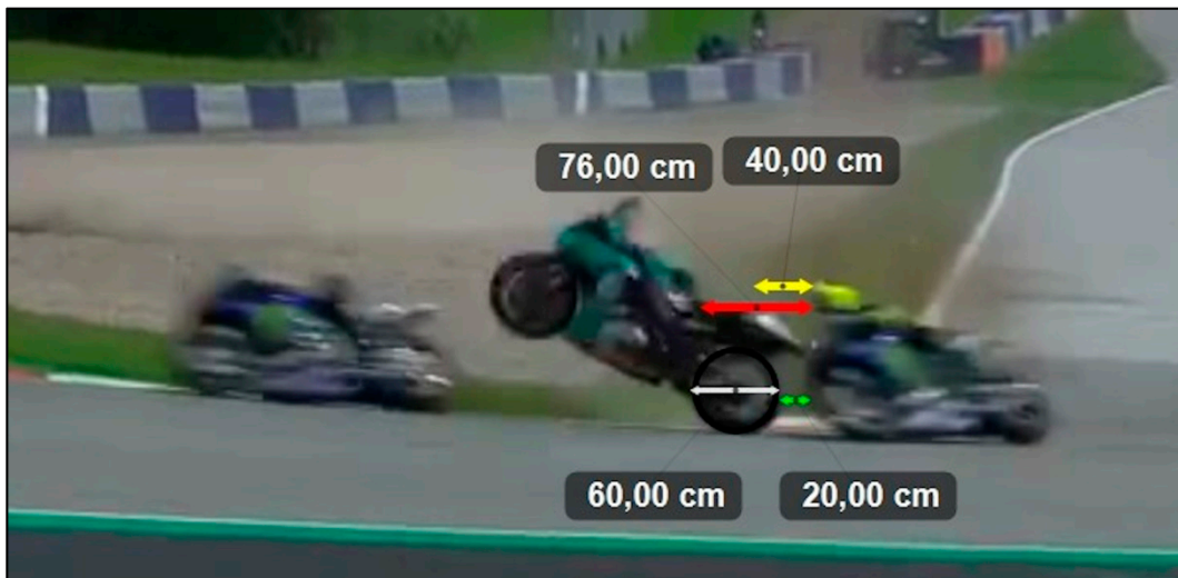
Figure 10. The frame capturing the exact instant when Morbidelli's bike crossed Rossi's path. Kinovea was used to measure the distances based on the measurement of the rear wheel of Morbidelli's bike. Specifically, the white arrows indicate the 60-cm diameter of Morbidelli's rear wheel (black circle); the green arrows represent the exact distance between Rossi's front wheel and Morbidelli's rear wheel; the yellow and red arrows indicate the distance that Rossi's bike would have covered if he had slowed down according to scenario 1 (about 40 cm) and scenario 2 (about 76 cm), respectively.
