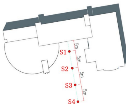
Figure 17. Setting of the measuring points near the building thermal interface.
